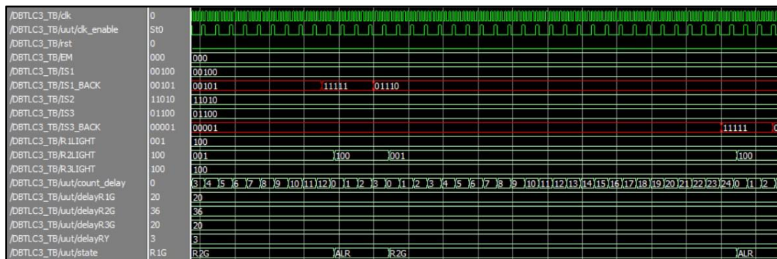
Fig. 11. The timing diagram for the real-time density-based traffic system with road blockage signal.
