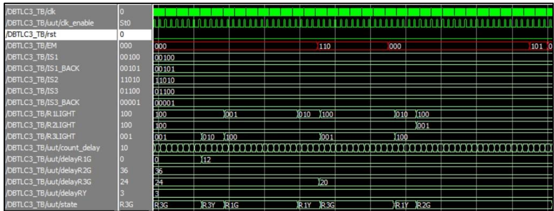
Fig. 12. The timing diagram for the real-time density-based traffic system with an emergency vehicle on road3.
